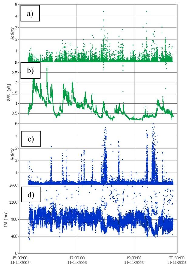
Figure 3 Typical output of emotion measurement platform: a) wrist activity b) skin conductance c) torso activity d) heart rate variability.
