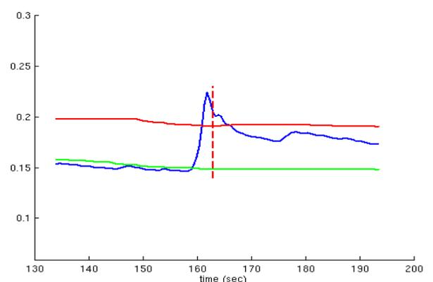
Figure 5: Screenshot showing the skin conductance signal (blue) and dynamic thresholds (red and green) and a trigger (vertical dashed line).
