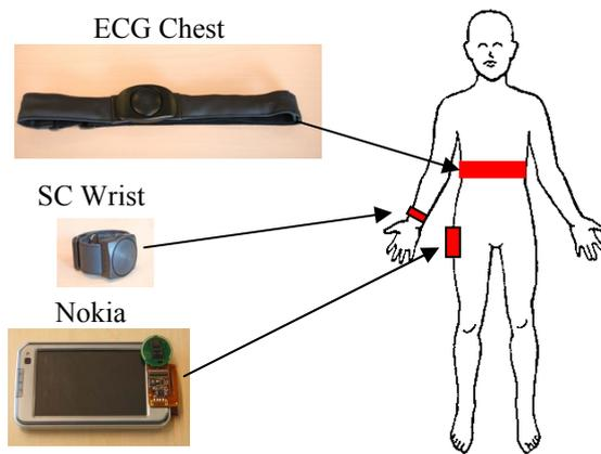
Figure 1: Elements of the Emotion Measurement Platform.
