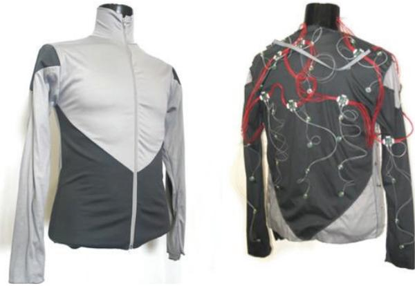
Figure 1: Outer lining (left) and jacket turned inside-out showing the inner lining with electronics and wires (right).
